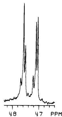
Figure 3. ^1\text{H} -decoupled ^{13}\text{C} NMR spectrum of C(7) (downfield) and C(1) in the product mixture from chloro olefin 10 . Each carbon has singlet peaks for environments with 0, 1, or 2 deuterium atoms on adjacent carbons.
